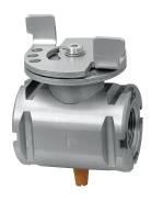
Ball / Lockout Valve shuts off downstream line pressure in the closed position with a 90° turn of the handle. In the closed position, inlet air pressure is blocked and downstream / system air is exhausted through a threaded port. To prevent unauthorized adjustment, the padlock slide may be assembled on either side. It is recommended that this slide is installed after final system assembly.
