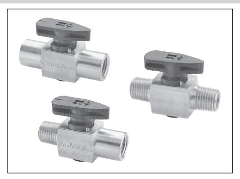
Compact design features internal nitrile seals and a one-piece extruded brass body, offering compatibility with a wide range of media. The one-piece stem / handle combination is constructed of glass reinforced acetal copolymer. Parker plug valves feature 1/4 turn shutoff allowing for ease of operation. All plug valves are 100% leak tested and are certified to be leak free to one SCCM.
