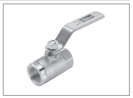
Parker's industrial ball valve product line is intended for general purpose use. Please be aware that ball valves are intended for use in the fully open or closed positions. Depending on application conditions, throttling of the valve may result in premature seal failure and/or inability to turn the valve handle.
