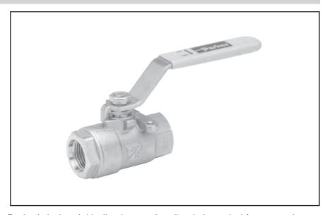
Parker's industrial ball valve product line is intended for general purpose use. Please be aware that ball valves are intended for use in the fully open or closed positions. Depending on application conditions, throttling of the valve may result in premature seal failure and / or inability to turn the valve handle.
