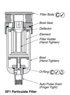
(A) Lightly grease with provided lubricant.
