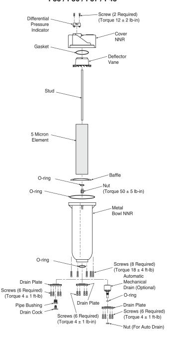
Automatic Mechanical Float Drain
