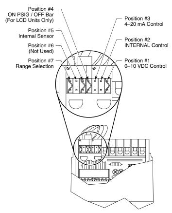
Figure 2 – Jumper Connections
