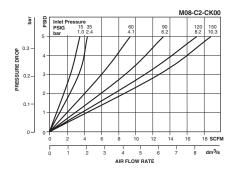
Flow data based on inlet pressure = 10.3 bar, .20 bar
