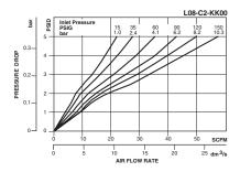
Flow data based on inlet pressure = 10.3 bar, .34 bar
